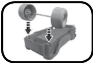
7. Attach the Pull Cart Back Support Pieces to the sides of the Pull Cart Seat. Insert the Pull Cart Back Support Pieces and the Pull Cart Front Support into the base of the Pull Cart until you hear them click into place. Once you have assembled the Pull Cart, it cannot be taken apart.
